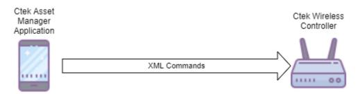
If your Wireless Controller is on a VPN, your device will need to have a VPN client enabled when sending XML commands.
